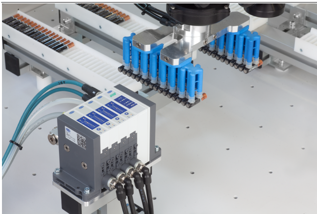
Compact terminal SCTSi Ethernet in the handling of batteries
